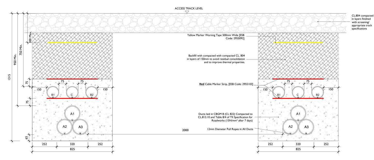
A = 160mm: Outer Diameter HDPE ESB Approved Duct, SDR= 21.0 (Power) [ESB Code: 9317560]
